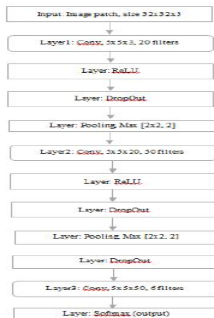
Fig. 7 Deep Convolutional Neural Network Model 1
