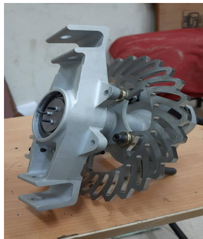
Fig.22 : Manufactured front wheel assembly
