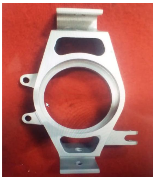
Fig.25 : Manufactured rear knuckle
