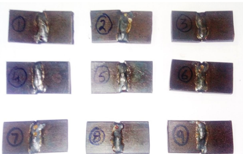
Fig. 1: MIG welded specimens
