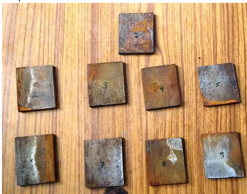
Fig. 1: AISI 1018 Specimens after corrosion test
