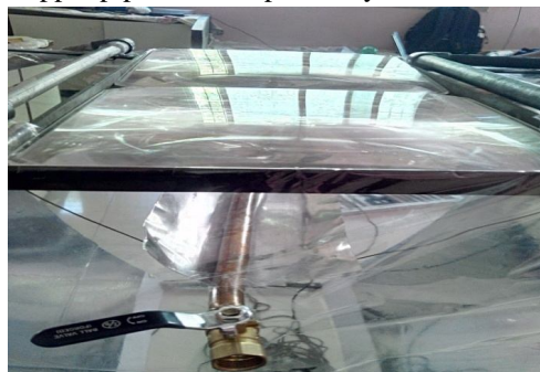
Fig.2 Assembly of Fresnel lens and copper pipe
