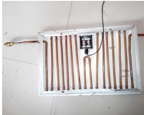
Fig.3 PV panel with heat exchange
