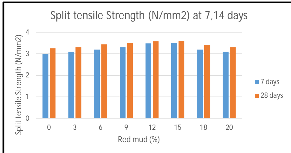
Graph 3: Effect of Red Mud on Split Tensile Strength of Different Mix of M-30 Concrete at 7&28 days
