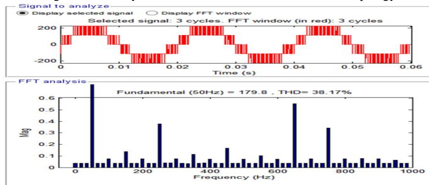
Fig. 21 FFT analysis for T-type topology of output voltage before filter
