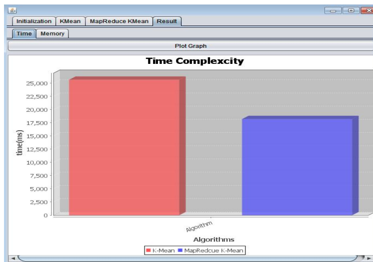
Fig 3: Comparison graph of time complexities Of K mean and Map Reduce K mean
