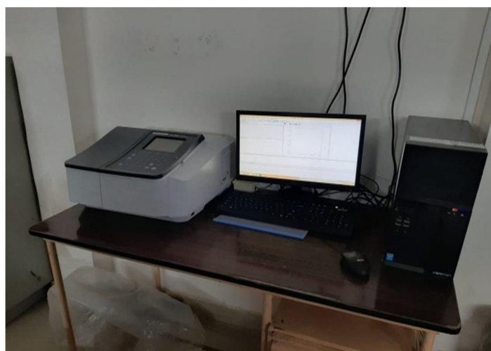
Fig.4 (b) UV-1800 SPECTROPHOTOMETER ALONG WITH PC CONTROL
