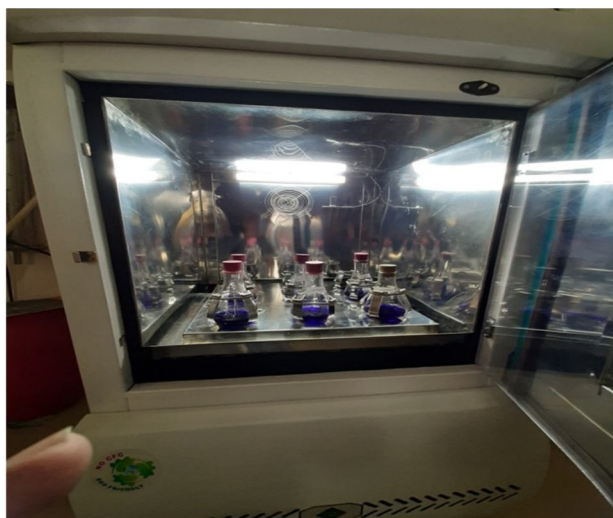
Fig.5 (c) Placing of sample in shaking Incubator
