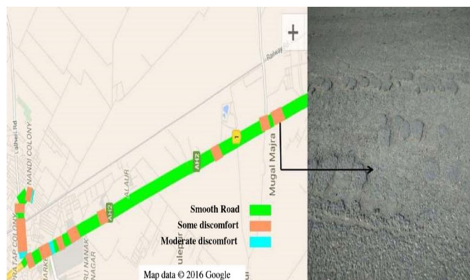
Fig.19 Road segment with some patches of discomfort (map data © Google 2016; image by Rajiv Kumar). Reproduced with permission. Copyright 2016, ASCE.
