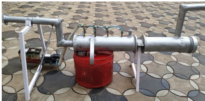
Figure 5 Aqua exhaust test rig (Atomization Method)
