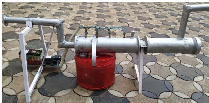
Figure 5 Aqua exhaust test rig (Atomization Method)
