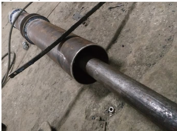
Figure 4 Aqua exhaust test rig (Normal Method)
