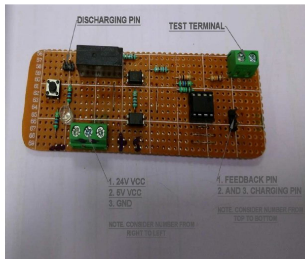
Figure 5 Top View of Current Triggering Circuit
