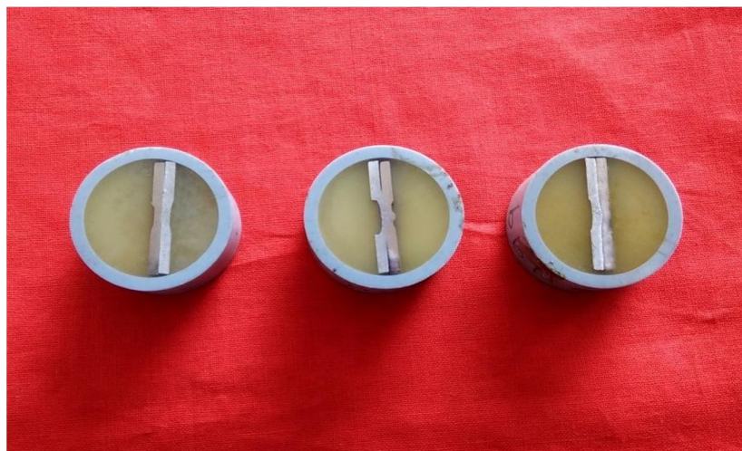
Figure 7.4 (a) Photographic view of microhardness samples of AIS5052 similar joints
