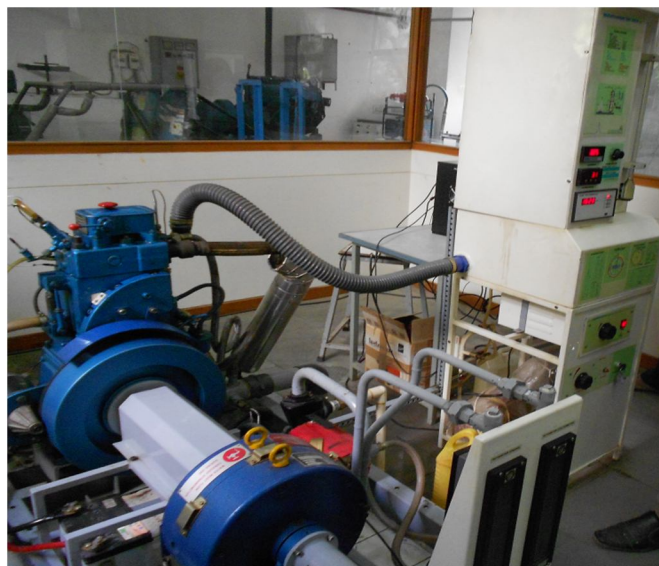
Fig. 3 Single Cylinder Diesel Engine Test rig
