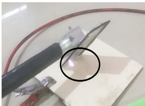
Fig10. Holiday present on the surface where coating is done.
