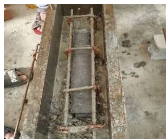
Fig. 9 Beam placed with 40 cm SRWT mould and shear reinforcement
