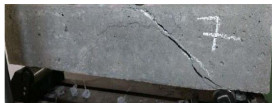
Fig. 5 Beam reinforcement without SRWT mould
