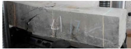
Fig.10 failure pattern on beam with SRWT mesh and shear reinforcement
