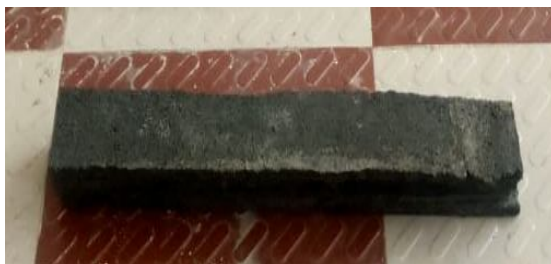
Fig 2 waste shredded rubber mould.
