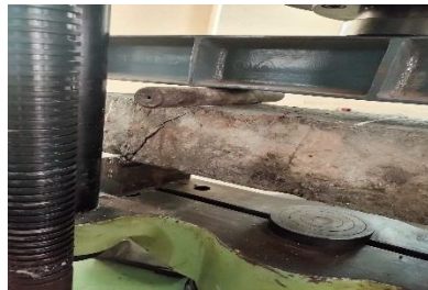
Fig. 7 flexure test on beam without SRWT mould
