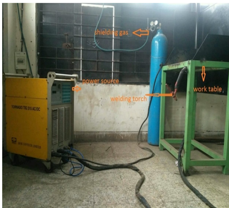
Fig. 1. Complete TIG welding set up
