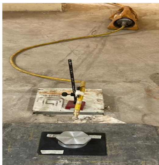
Fig.21 Radiography Testing Set-up
