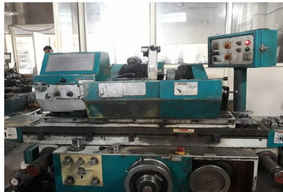
Figure.2.1 Setup Cylindrical Grinding Machine
