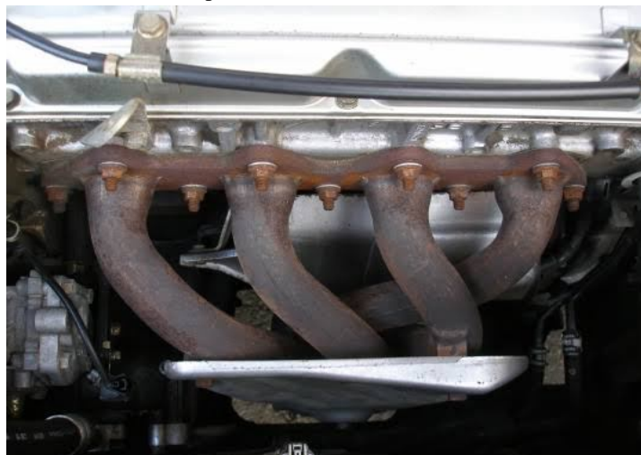
Fig.1 Engine- Exhaust manifold assembly
