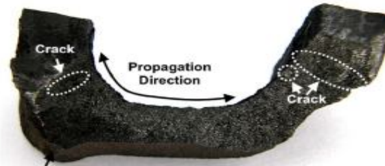
Fig.2 Crack development on runner
