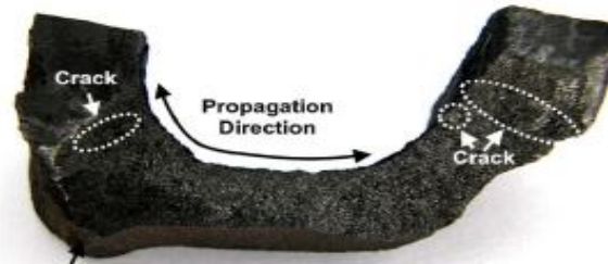
Fig.2 Crack development on runner
