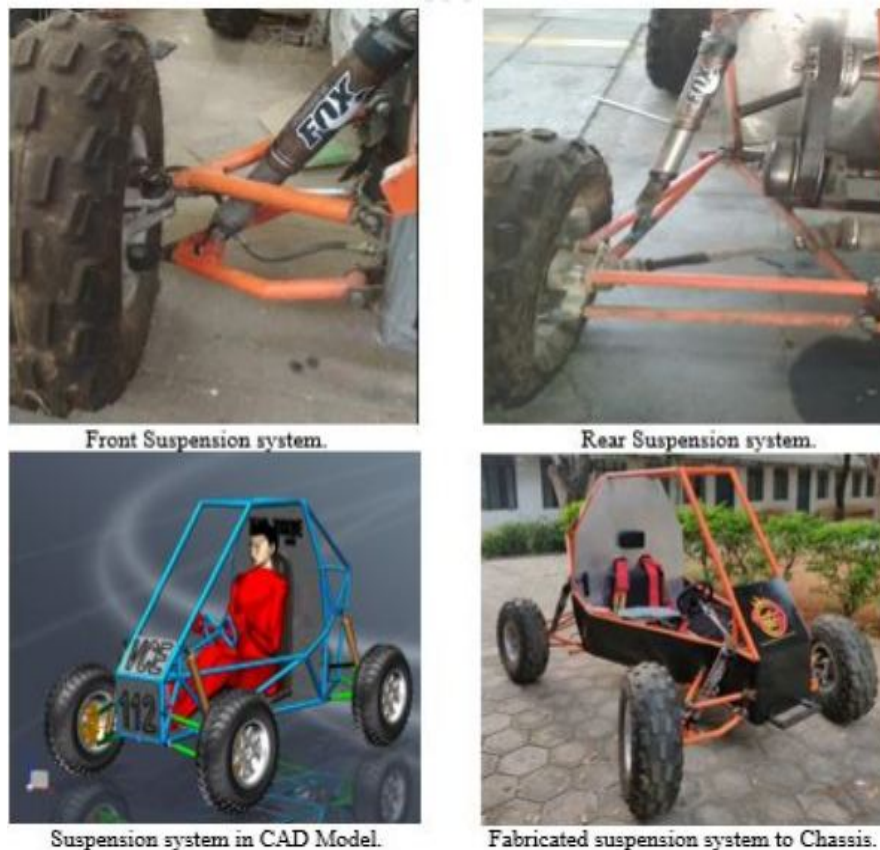
Figure 19: Assembled suspension system to the chassis.
