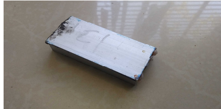
Fig 3: Heat sink without liquid cooling
