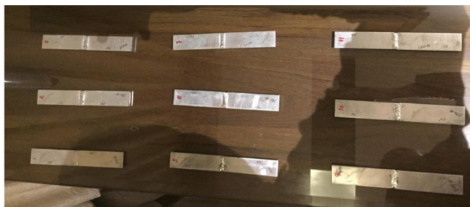
Fig 8 Prepared samples after welding
