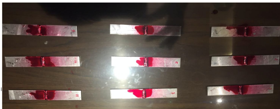
Fig 9 Samples after applying Dye penetrant
