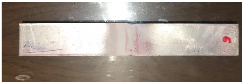
Fig 10 Sample after applying Developer
