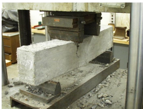
Figure 2 Flexural strength of steel fibre rice husk and rice husk ash beam after testing
