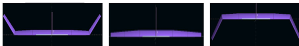
Fig. 2 Span morphing at +45°, 0° and -45°
