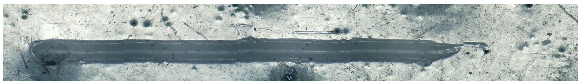
Figure 7: Scratch on the coating of 0 % reinforcement SiO 2
