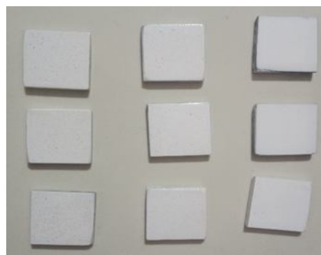
Figure 2: mild steel sample after coating
