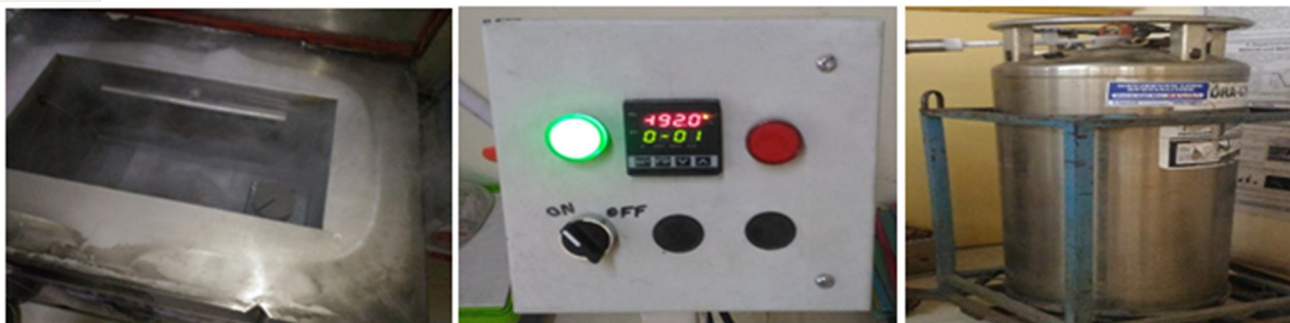
Figure 3 Cryogenic Chamber, Temperature Controller, Liquid Nitrogen tank
