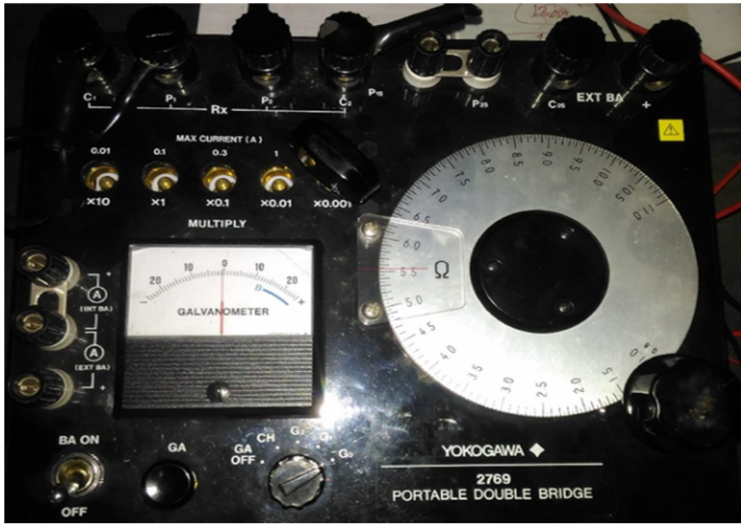
Figure 6 YOKOGAWA double bridge meter
