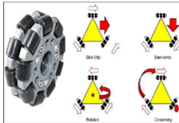
Fig. 2.2 The operation of a rotating three-wheeled type.
