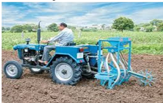
Fig.4. Malobansa way of seed dropping
