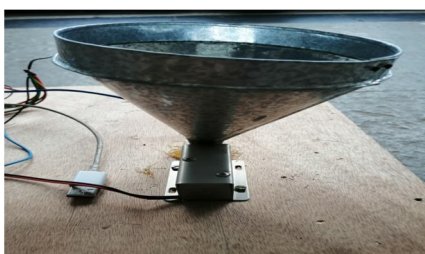
Fig.16. Solenoid Lock Coupled to a Funnel
