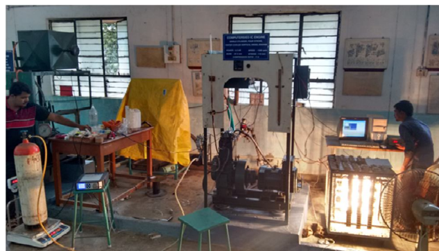
Figure II-3: Computerized, Electrical loading single cylinder four stroke CI engine converted to Dual fuel mode with compressed Biogas used as a fuel
