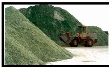
Crushed glass aggregate for concrete
