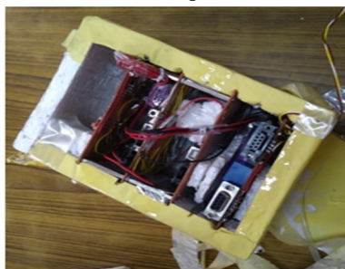
Fig 10. Cubesat Proto Model with stacked board
