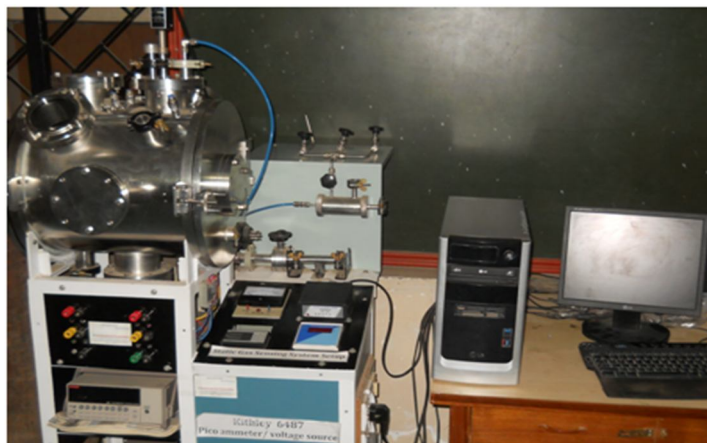
Fig. 1 Photograph of computerized gas sensing system
