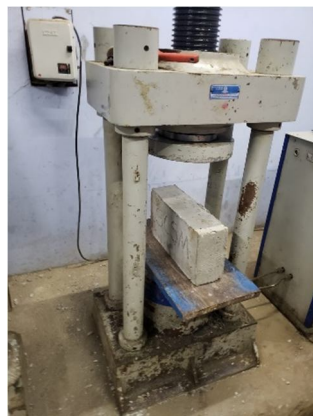
Clay bricks compressive strength is 2.2 kN/mm 2 to 2.3 kN/mm 2 .
