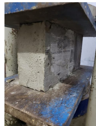
Clay bricks compressive strength is 2.2 kN/mm 2 to 2.3 kN/mm 2 .
