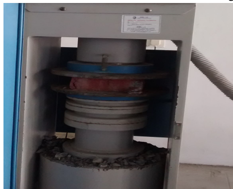
Fig. 3 Compressive strength test
