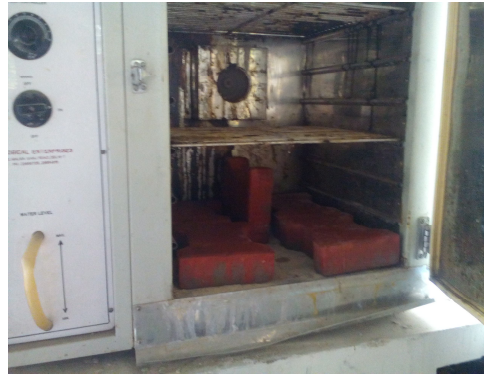
Fig. 2 Paver blocks in oven
