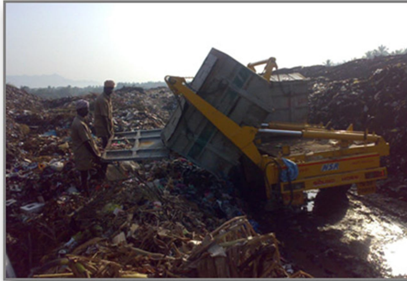
Fig.3.2.Secondary Collection Process by Using Tipper Lorry
