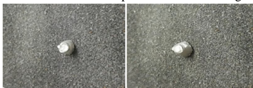
Fig.8. a)Pulsed AC fracture specimen and b) Pulsed DC fracture specimen(cup-cone)
