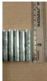
Fig. 1. Specimens after ECAP process
