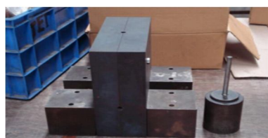
Fig. 2. Die used to do ECAP of specimens
