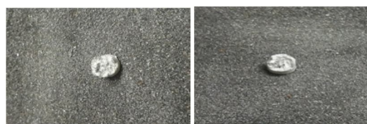
Fig.9. a)Constant AC fracture specimen and b) Constant DC fracture specimen(flat-fracture)
