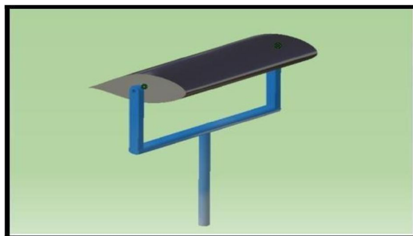
Figure 10: Clamping of aerofoil using a C-Clamp
