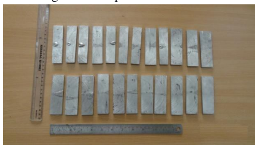
Figure 2: Samples before bend test
