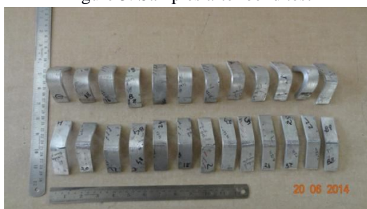
Figure 3: Samples after bend test
