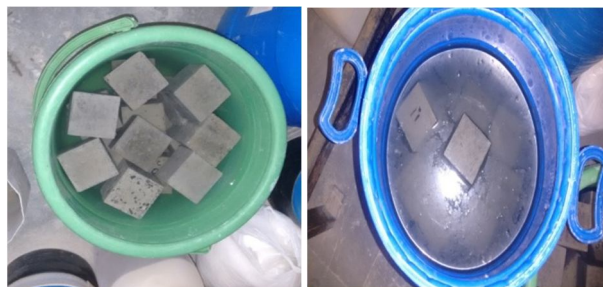
Sample placed in H_2SO_4 and Sodium Sulphate
