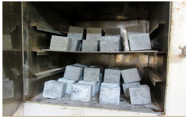
Oven curing of cubes
