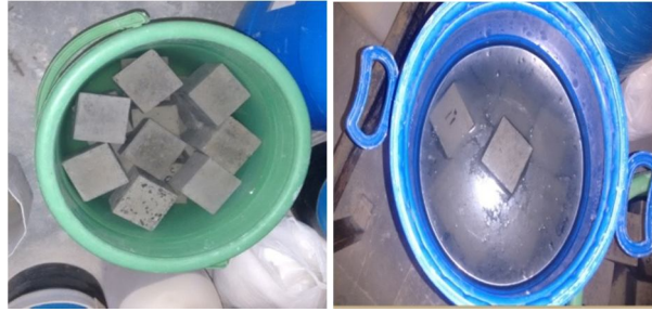
Sample placed in H_2SO_4 and Sodium Sulphate
