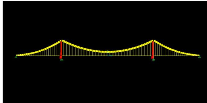
Fig. 24. Represents the axial forces being applied on the suspension bridge structure. The parts shown in yellow are the cable axial force diagram while the red representation shows the axial force on towers due to the cables.
