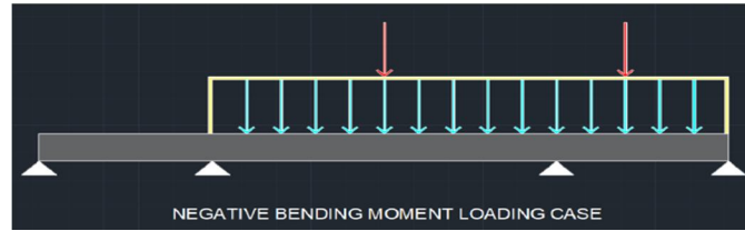
Fig. 5. Shows the loading of the deck with an eccentric uniform load which would give a negative bending moment; a hogging deck. This case shows the off-centre region of the bridge deck to have been loaded uniformly and as with the case of uniformly distributed load, here also the load acting has been considered as acting at respective proportions mid-point.
