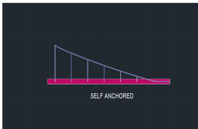
Fig. 27. Shows that the cables are anchored to the deck itself. This self-anchoring of the deck allows the region to have a lesser axial force and this is evident from table VII showing the decrease in axial force in the support region.
