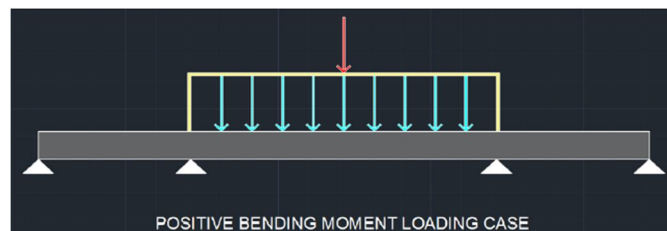
Fig. 4. Shows the loading of the deck with a uniform load which would give a positive bending moment; a sagging deck. This case shows the centre region of the bridge deck to have been loaded uniformly and as with the case of uniformly distributed load, here also the load acting has been considered as acting at centre.
