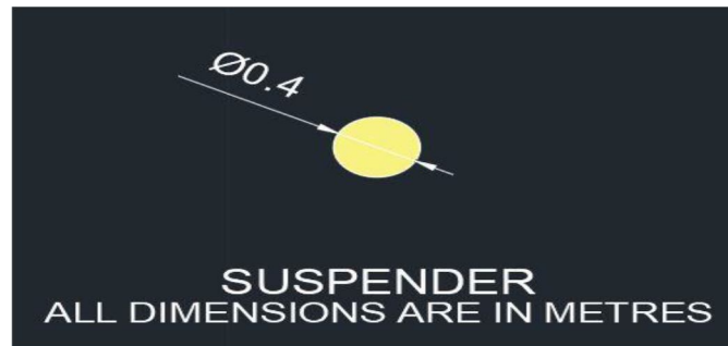
Fig. 21. Shows the suspender cross section of radius 0.2 m.
