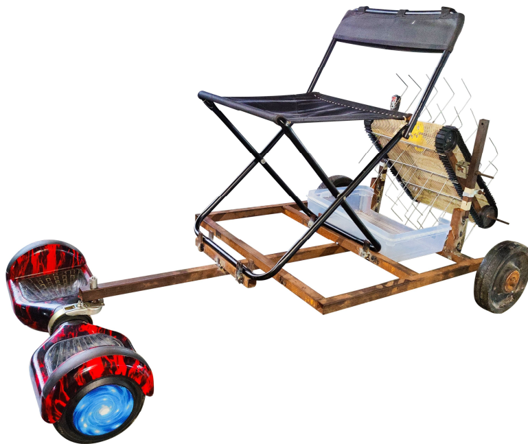
Fig. 1 Actual model of garbage collector and load transporting carting hoverboard vehical
