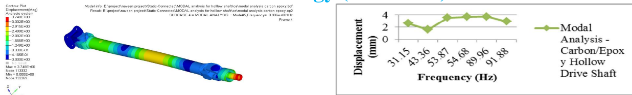
Fig. 6. Max Displacement result of modal analysis of hollow carbon/epoxy T700S drive shaft
