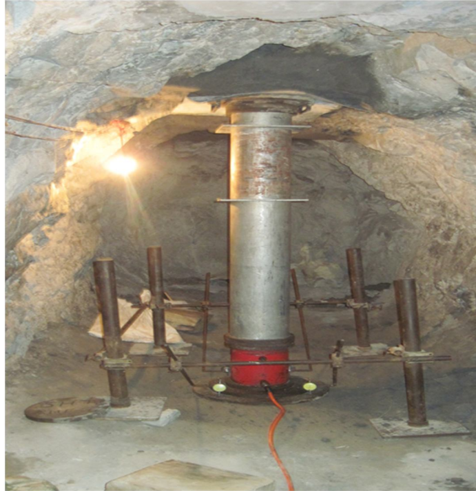
Fig. 3 In-situ Plate Load Test Setup
