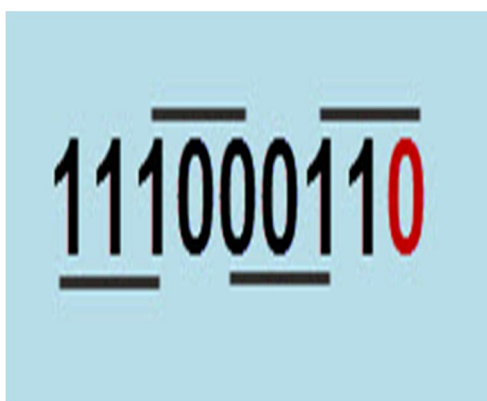
Fig. 2 3-bit pairing for Booth recoding
