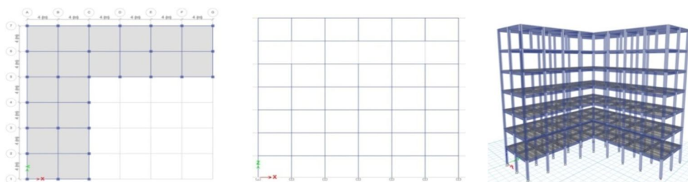
Fig.10 : Plan and section of L shape building with floating column at top middle
