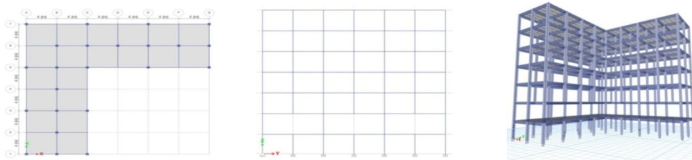
Fig.7: Plan and section of L shape building with floating column at bottom corner
