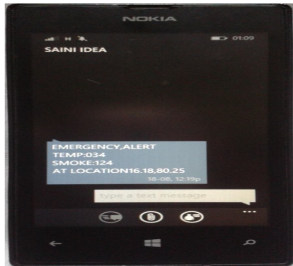
Fig5: Output values are displayed as a SMS using GSM technology
