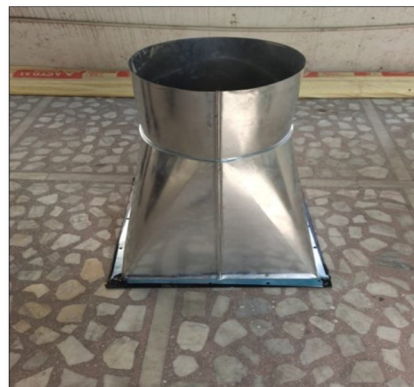
Fig 18: Convergent duct fabrication
