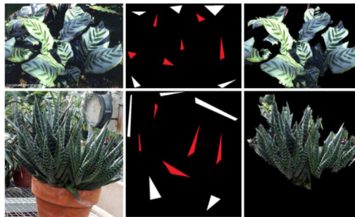
Fig 2.1: Segmentation examples the input image, the seed points shown as white (background) and red (foreground) regions and the segmented images are shown in a row.
