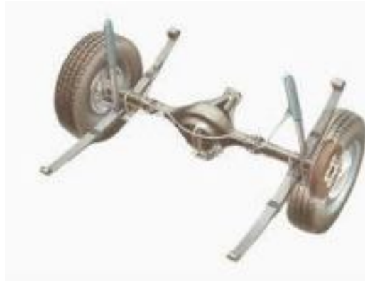
Fig: Setting the leaf spring in the model of a car
